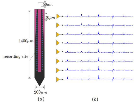
Fig. 2. a) Photomicrograph of a Polytrode. The shank has planar recording sites spanned 50  $\mu\text{m}$  apart in two columns. Polytrodes with denser site spacing provide highly detailed field recordings and span 1mm. [8] b) Signals recorded by sensors in a real experiment. The signals are closely correlated. The data is taken from the website <http://crcns.org>.
